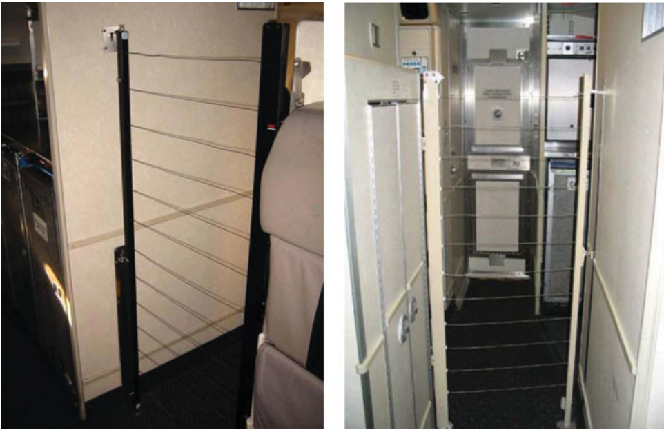
Figure 4. Fully Deployed Installed Physical Secondary Barrier.
