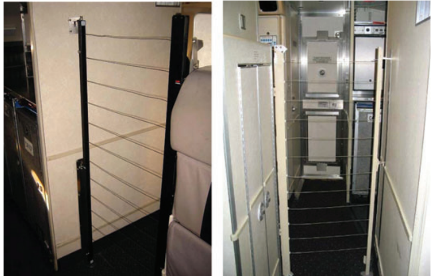
Fig. 2. Fully deployed installed physical secondary barrier. (52)
